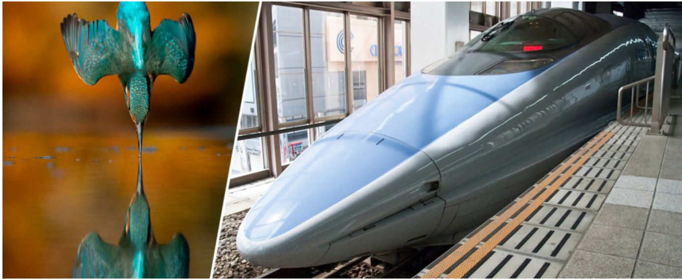
The kingfisher-like nose of a bullet train prevents sonic booms. (2019, agosto). [Fotografía]. ScienceABC. https://www.scienceabc.com/innovation/what-is-biomimicry-definition-real-life-examples.html
