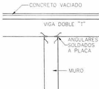
VIGAS DOBLE "T" Y MUROS
