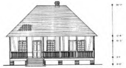
FRONT ELEVATION NOTES Base color scheme on white and red in French Corridor, entrance, hallway, kitchen, parlor and sleeping, red with; base color woodwork, exterior grey roof/shingles red asphalt
